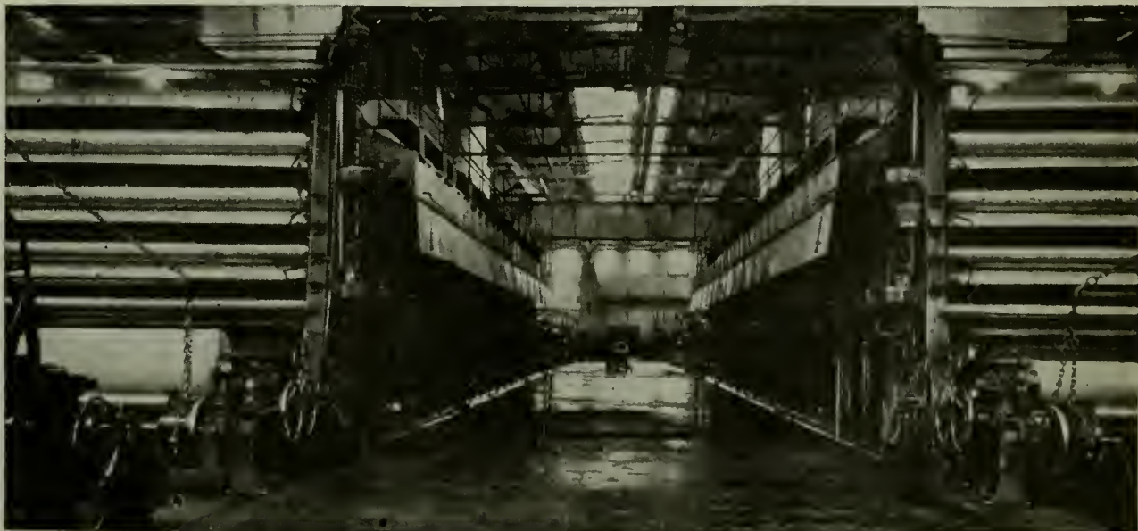
The "dry" end of the same machines. The sheet of paper coming from the machine is being rolled into a huge roll, and the chains will carry it to the finishing-room.
